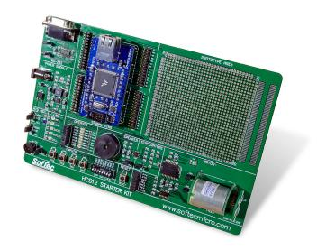
The AK-S12NE64-A Starter Kit is an integrated system designed to provide the user with a complete, ready-to-use embedded Ethernet application. The Starter Kit is built around the Freescale MC9S12NE64 microcontroller, which has a built-in, dedicated Ethernet peripheral. The Starter Kit demonstrates how effectively the MC9S12NE family of microcontrollers can be used in real-world embedded Ethernet applications.
